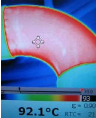
Thermal imaging shows the surface temperature of uninsulated piping (left) reduced by about half with 6 mm of Pyrogel 6350 aerogel insulation (center). Photo at right shows fully insulated section of piping with elbows.
